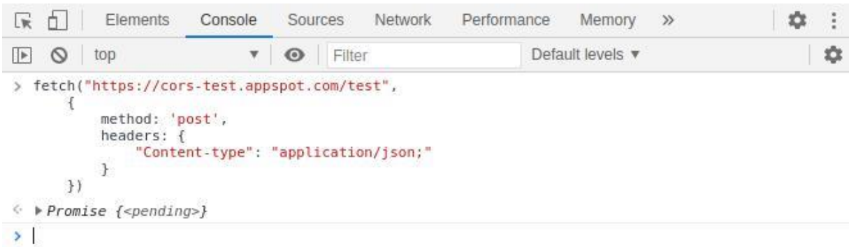
Figure 289: POST Request with Non-Standard Content Type With CORS Response
